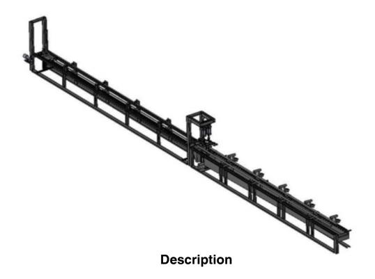
Installation of mechanical cleaning of the inner surface of pump-compressor pipes is designed to clean the internal surface of pump compressor pipes from solid operational deposits.
